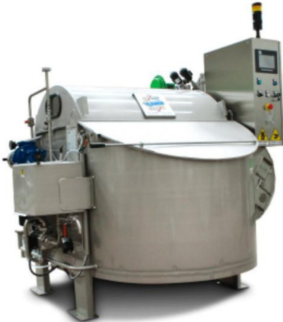
Figure 1 - Hollander-type paddle machine for garment dyeing
